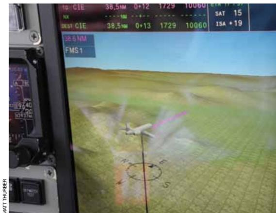
Universal Avionics, which was an early adopter of synthetic vision technology on its EFI-890 display, offers pilots an exocentric view that is also an accurate representation of the aircraft's attitude. Could such a view help show that the aircraft is in a stall?
