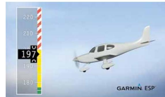
Garmin's ESP works with the autopilot on or off and assists the pilot in maintaining a safe pitch and roll attitude and airspeed, including low-speed protection.
